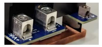
AC output voltage is connected via cable to three power lugs on the AC-output side of the drive.
